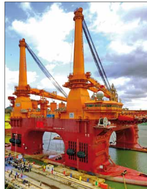
The deepwater semi-submersible crane and accommodation vessel delivered to Petrobras by Yantai CIMC Raffles Offshore Ltd Co
